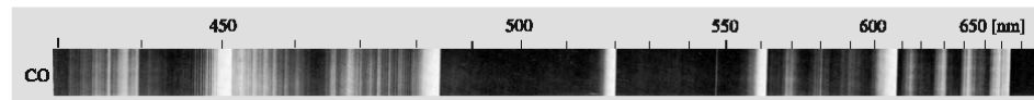
Fig. 5.9. Spectrum of carbon monoxide CO from 430 nm to 670 nm. The various bands correspond to different vibrational transitions. Each band is composed of numerous rotational lines. Near the right edge of each band the lines are so closely
