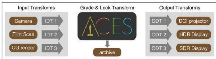
An ACES imaging path from the Cinematographer Quick Start Guide (QSG), part of the ACES Subcommittee section.
