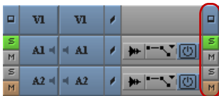
Track Selection panel, with video and audio tracks selected for solo monitoring
