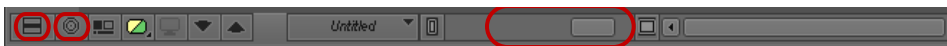
Left to right: Timeline Fast Menu button, Focus button, and scale bar in the Timeline bottom toolbar
