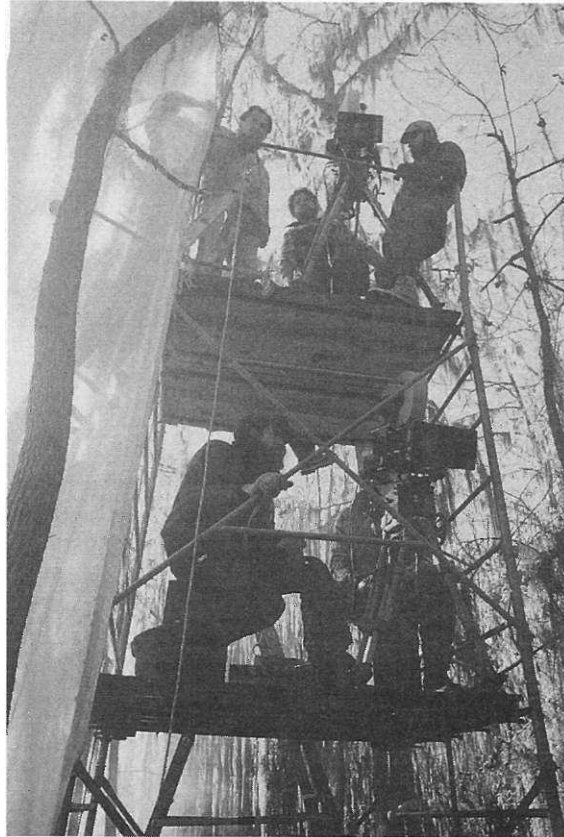
Figure 1.9 A multiple camera set up on a parallel. Note silk panel and smoke
