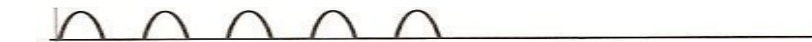
combination of half-wave rectified AC (1s or 1.2s) and pause (1s or 1.2 s)
